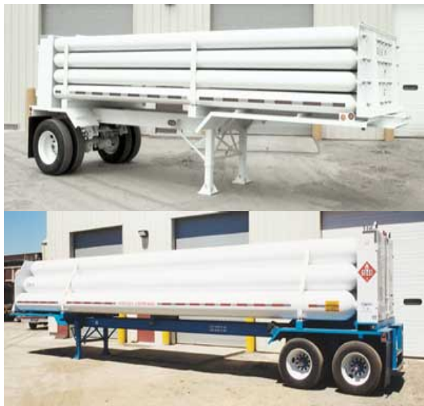
Figure 7. Standard and Jumbo Hydrogen Tube Trailers Source: Weldship
