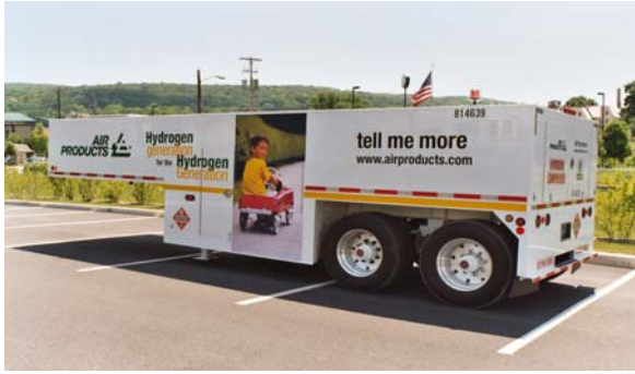
Figure 9. Air Products 150 kg Mobile Hydrogen Fueler Source: Air Products
