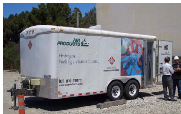
Figure 8. Air Products 50 kg Mobile Hydrogen Fueler Source: Air Products
